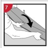
Second plank, second row: Place the short end of the plank at an angle against the previous installed plank and fold down.
