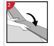
Second plank, first row: Press the short end of the next plank at an angle to the first one, and then fold down. Complete the first row with the same method.
