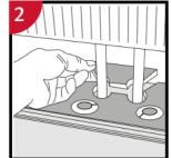
When angling is not possible: Remove the vertical locking part of the strip with a chisel, put applicable glue on the strip and push the planks horizontally together. Use spacers between last board and wall.
