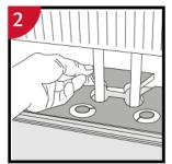
When angling is not possible: Remove the vertical locking part of the strip with a chisel, put applicable glue on the strip and push the planks horizontally together. Use spacers between last board and wall.
