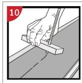
Last row (and perhaps also first row): Always keep a minimum width of 2". Place a spacer to the wall before measuring. Mark the plank along the wall. Cut the planks lengthwise including the flexible tongues and install.
